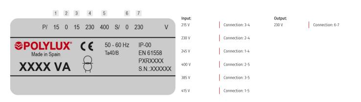
Single phase dry type isolation transformers, finished in IP00 anti-flash varnished with protection to prevent direct contact with electrical parts.
