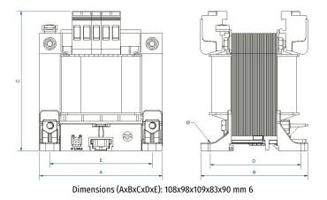
Single phase dry type isolation transformers, finished in IP00 anti-flash varnished with protection to prevent direct contact with electrical parts.
