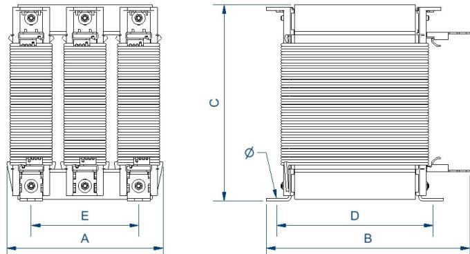
Three-phase line reactors for harmonic filtering with bimetal over-temperature protection resin finished and anti-flash varnished.
